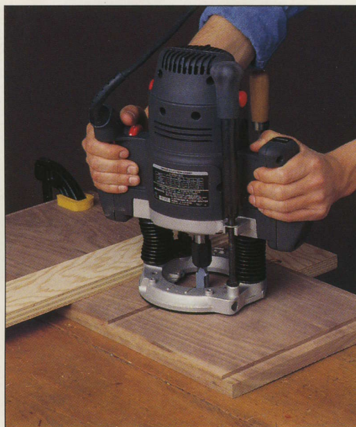
Shelves are often fixed to carcass sides with dado joints. Here, a router plows a through dado. An edge guide helps keep the cut parallel to the end of the panel.
