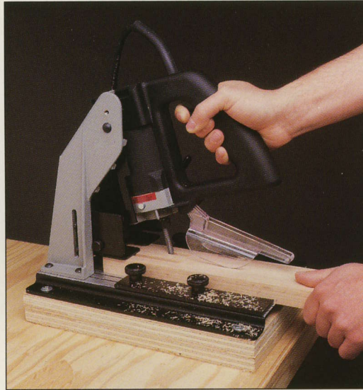
The commercial jig shown above cuts accurate pocket holes with a minimum of setup time. With the workpiece clamped in the jig, the router-like cutter is pivoted into the face of the board to cut the pocket hole.
