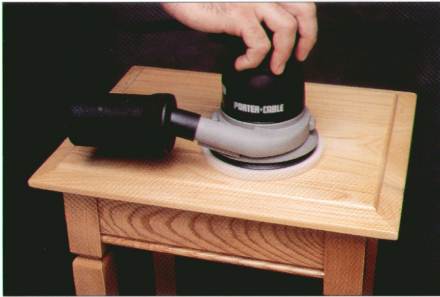
Fitted with a lamb's wool buffing bonnet, a random-orbit sander serves as an electric polisher, rubbing out the finish and buffing the topcoat to a high-gloss sheen.
