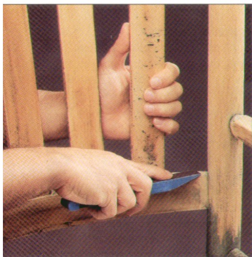
A sanding stick smooths the back rail of a chair. This device is ideal for reaching into tight spots, such as the spaces between the slats of a backrest.
