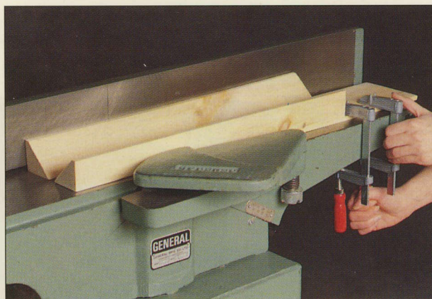
With a V-block jig clamped to the jointer infeed table, you can cut beveled edges into a workpiece accurately and safely.
