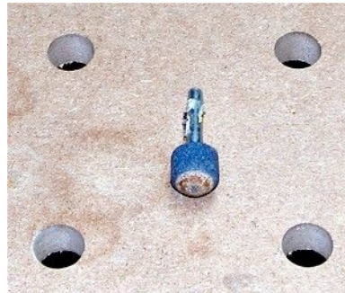
Cedar sides were attached to the with a dowel glued into each board. Then the game board was sanded. The special drill bit to the right was used to sand the marble indents.
