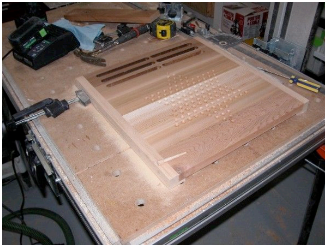
Cedar sides were attached to the with a dowel glued into each board. Then the game board was sanded. The special drill bit to the right was used to sand the marble indents.
