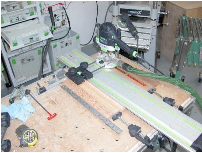
Routing grooves into the board
