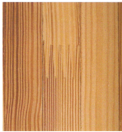
Figure 16.4 • Glulam is a stress-rated product made up of two or more layers of lumber glued together with their grain directions parallel to one another. This is a finger joint in a lamination of glulam decking (shown in Figure 16.5, top center). (Photo by Randy O'Rourke)
