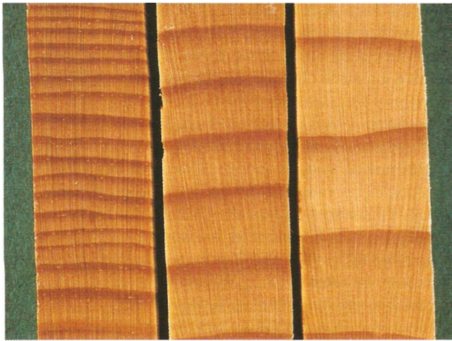
Figure 4.50 • In softwoods, the slower the growth, the stronger the wood. The variable rate of growth in red pine is shown here by the spacing of growth rings. The narrower the earlywood band, the stronger the wood. (Photo by Randy O'Rourke)
