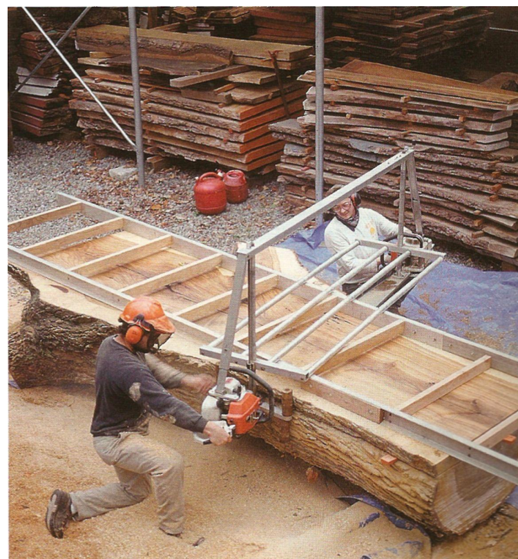
Figure 17.2 • The chain saw mill produces boards from a log. (Photo by Vincent Laurence)
