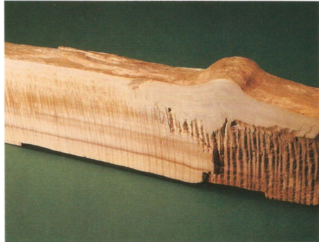
Figure 2.10 • Curly figure results when longitudinal cell structure forms a wavy pattern. When the wood is split, a washboard surface results. Curly figure is most pronounced when cut radially, as in this sugar maple. (Photo by Randy O'Rourke)
