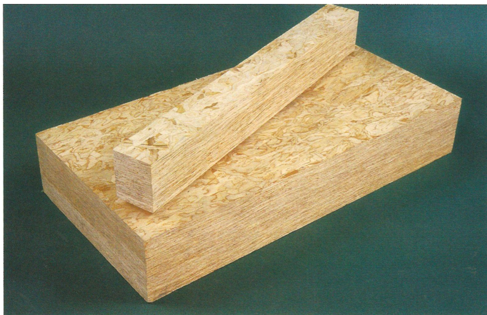
Figure 16.9 • A large slab of laminated strand lumber, prior to cutting into parts for framing upholstered furniture. The strands are bonded with isocyanate adhesive and cured with steam, which also makes the wood denser. (Photo by Randy O'Rourke)
