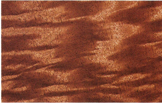
Figure 2.17 • Mottled figure occurs when the curly figure predominates in a piece with a combination of wavy and interlocked grain. (Photo by R. Bruce Hoadley)
