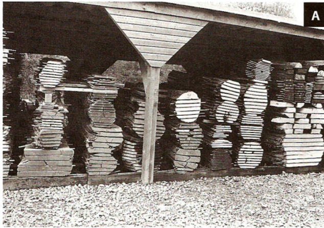
Figure 8.11 • Most of the boards in the drying shed (A) are restrained by the weight of the others. A similar but simpler setup (B) uses a sheet of corrugated plastic to protect the wood. In both cases, the boards are stacked in the sequence they came off the saw. (Photos by Richard Starr)
