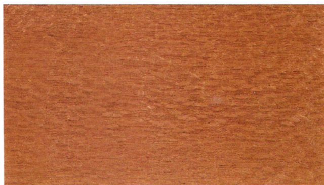
Figure 2.4 • Lacewood with ray fleck figure. This piece was rift-cut just off the true radial to produce interesting figure while reducing the size of the flecks. (Photo by Randy O'Rourke)
