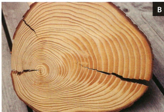
Figure 2.36 • Reaction wood forms in trees that lean (A). The curving sweep of this hemlock tree, although picturesque, means unpredictable compression wood will be found within as shown in the cross section (B). The section of spruce (C) shows severe compressive wood formation. (Photo A by R. Bruce Hoadley; photos B and C by Randy O'Rourke)
