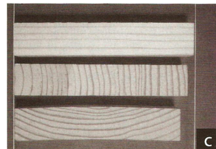
Figure 6.7 • Each photo shows a longitudinal (top), radial (center), and tangential (bottom) strip of wood, equal in length when green. (Photos A and B by R. Bruce Hoadley; photos C, D, and E by Randy O'Rourke)
