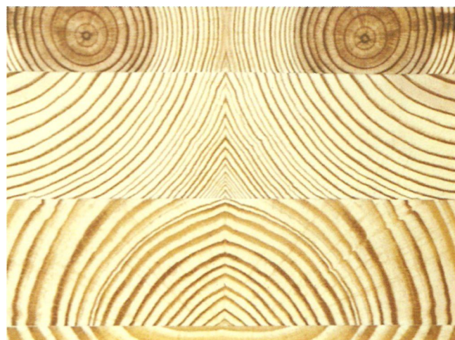
Figure 1.7 • Each growth ring in southern yellow pine is distinct, showing a light, soft layer of earlywood followed by a darker, denser layer of latewood. The visual contrast between earlywood and latewood predicts a corresponding difference in hardness of the wood. (Photo by R. Bruce Hoadley)
