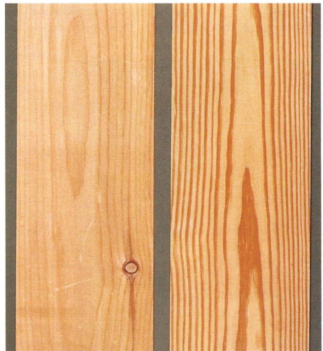
Figure 1.8 • Uneven-grained woods like southern yellow pine (right) have visually prominent rings. In fairly even-grained woods like eastern white pine (left), the contrast between earlywood and latewood is not as pronounced. (Photo by Randy O'Rourke)
