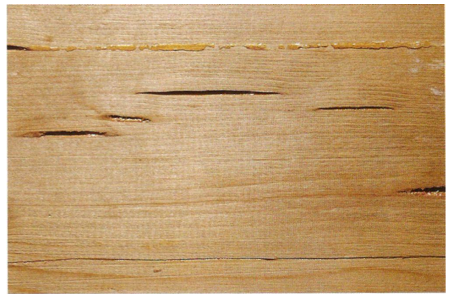
Figure 1.21 • Pitch pockets in a spruce board. Pitch pockets are lens-shaped voids filled with resin, which sometimes occur in woods having resin canals. (Photo by R. Bruce Hoadley)
