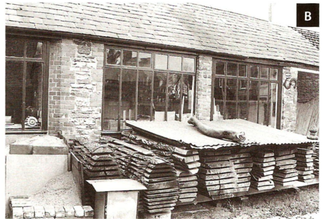
Figure 8.11 • Most of the boards in the drying shed (A) are restrained by the weight of the others. A similar but simpler setup (B) uses a sheet of corrugated plastic to protect the wood. In both cases, the boards are stacked in the sequence they came off the saw. (Photos by Richard Starr)
