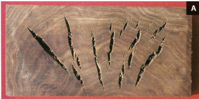
Figure 8.4 • Honeycomb checks in a black walnut plank follow the planes of the rays (A). Honeycombing in a maple square (B). Surface planing reveals the honeycombing in an oak board (C). (Photos A and C by R. Bruce Hoadley; photo B by Randy O'Rourke)
