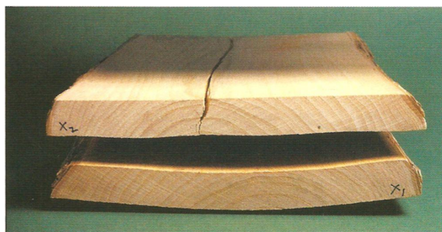
Figure 6.18 • Half of a cupped elm board (top) was flattened and cracked by the pressure of the rollers in a thickness planer. The other half exhibits the original cup. (Photo by Randy O'Rourke)
