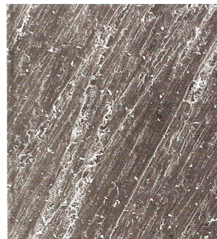
Figure 12.4 • The sample sanded with 220-grit paper looks much like the scraped surface, although there are more visible scratches. Dust, rather than torn fibers, seems to have filled the open vessels. A surface like this would feel quite smooth to the touch. 50X magnification. (Photo by Stephen Smulski)
