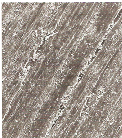
Figure 12.3 • When the surface is scraped with a steel scraper blade, torn and rolled wood tissue fills most of the wood vessels, and the surface becomes scratched by the minute ruggedness of the scraper's edge. 50X magnification. (Photo by Stephen Smulski)
